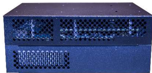
Figure 6. Left side – Convection air exhausts
