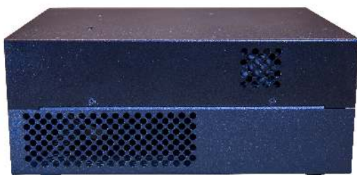
Figure 5. Right side – Convection air intakes
