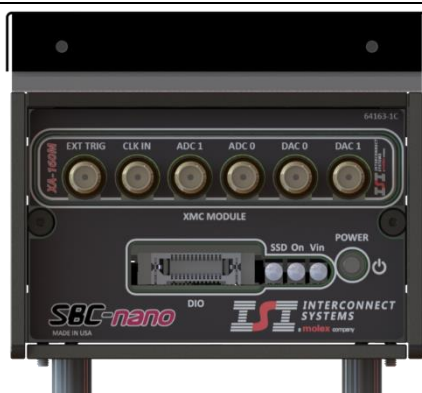
Figure 2. Front view of SBC-Nano system in a chassis with XMC module installed. Fansink (on the top) can be substituted with a coldplate in conduction-cooled applications.
